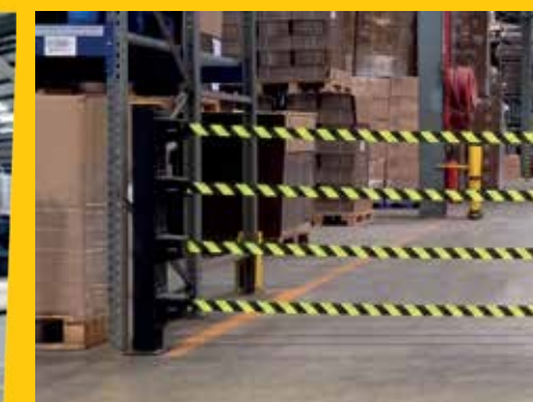
Highly visible tape to cordon off hazardous areas.
