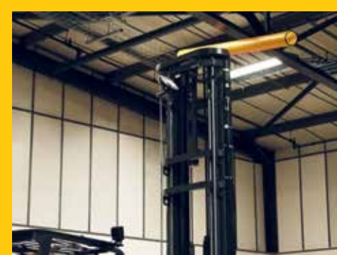
The Alarm Bar providing a visual alert to a vehicle driver.
