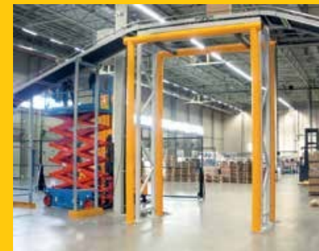
Bespoke height protection designs for overhead walkways and conveyors.
